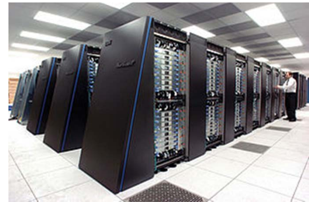
IBM's Blue Gene: 250,000 processors in 72 racks
